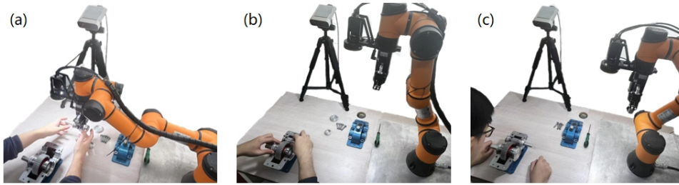
Figure 5: Action samples of the operator and robotic arm. (a) Selecting parts; (b) assembling parts; (c) checking.
