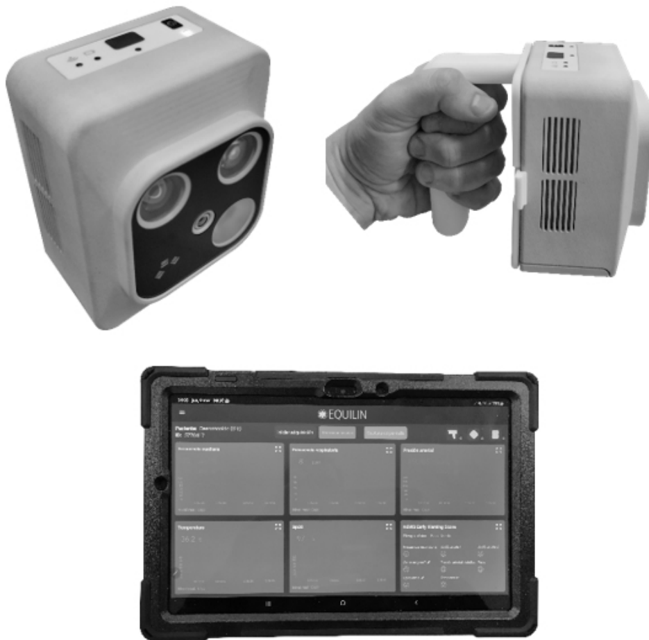
Figure 1: EQUILIN TRL 7 prototype: remote PPG device and dashboard user interface.
