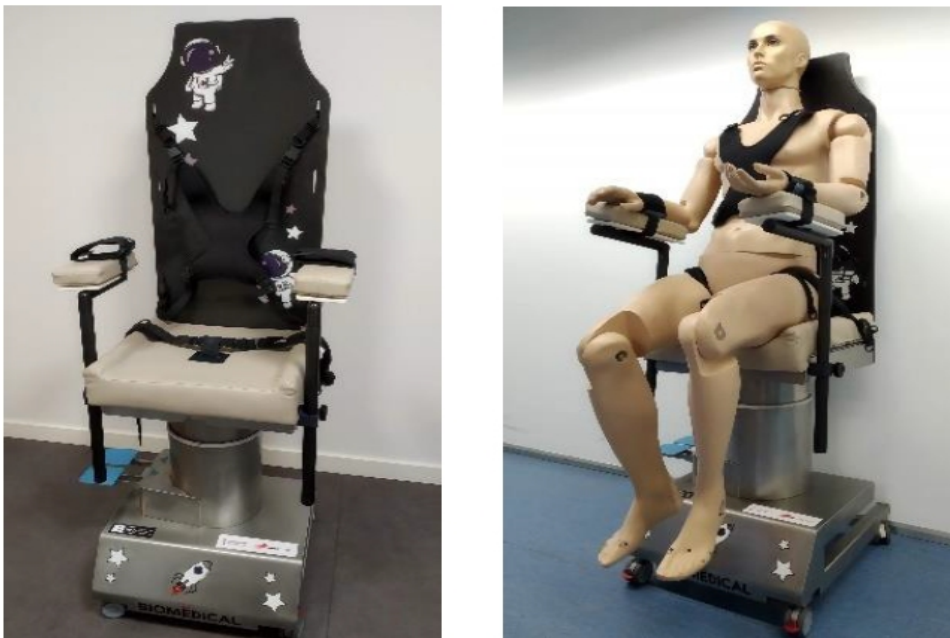
Figure 7: Functional prototype of the imaging sitting support device of Eiffage.
