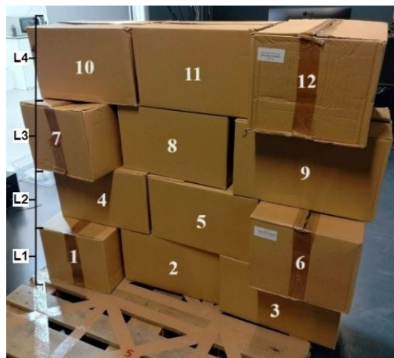
Figure 1: Scheme and sequence of deposit of the boxes on the four levels (L1, L2, L3, L4) on the pallet.
