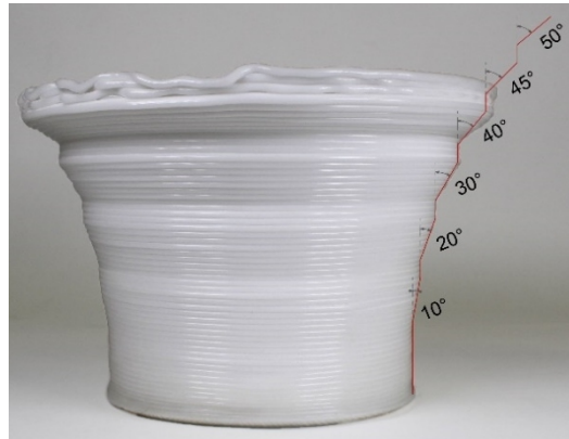
Figure 2: Resulting first sample-part at different angles with section delineation of each expected angle outcome.
