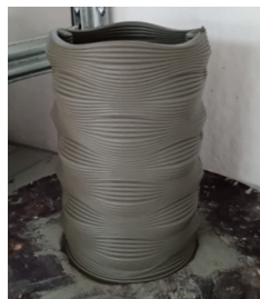
Figure 7: Materia project. Detail of the surface of the vase in the prototyping phase through ceramic 3D extrusion printing at WASP (source: WASP – 3dwasp.com).
