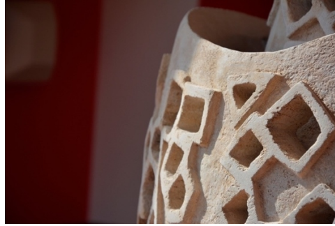
Figure 1: Desamanera “pelle di pietra” project, created by powder-based technologies.
