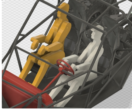
Figure 3: Scaled manikins (yellow and white) of one of the teams, sitting down in the ATV (gray). The steering wheel and its base (in red) were designed with a telescopic support to account for both manikins.
