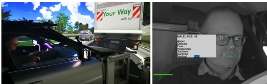
Figure 2: Standstill after the automated approach at a distance of 3m behind the truck (left) and emotion analysis by the Visage FaceTrack and FaceAnalysis SDK v9.0 (right).
