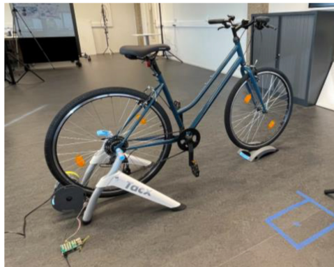
Figure 3: The virtual reality cycling simulator.
