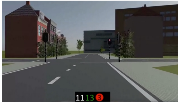
Figure 2: Driving simulator scenario with eco-driving interface. On the left of the interface, it displayed drivers' current driving speed (in mph). In the middle, it shows the suggested speed (in mph). If the suggested speed was larger than the driver's current speed, it would be shown in green color. Otherwise, it would be shown in red color. On the right-hand side of the interface, it was a color state of the current traffic light with a timer indicating the remaining time of the current state.
