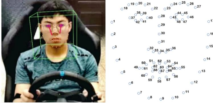
**Figure 2:** Detection of facial landmarks.
