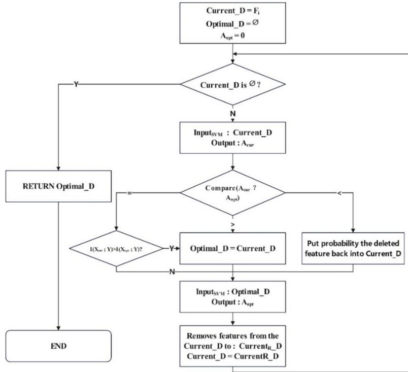
**Figure 4:** Flowchart of the C-SVM-RFE algorithm.
