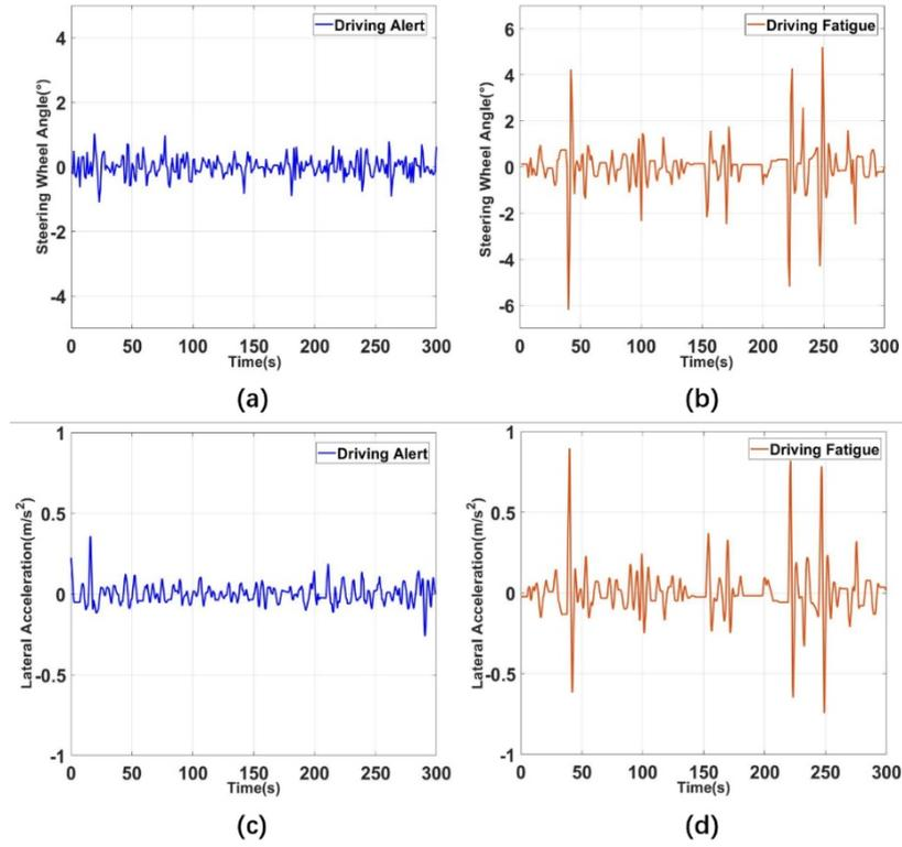
**Figure 3:** Trends of steering wheel angle and vehicle lateral acceleration under different driving conditions.
