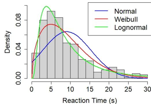
**Figure 2:** Histogram of the reaction times and the fitting curves of three different distributions.
