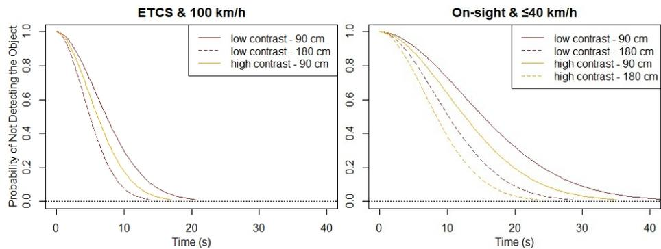
**Figure 4:** Survival probabilities in ETCS at 100 km/h and in on-sight-driving at 40 km/h.
