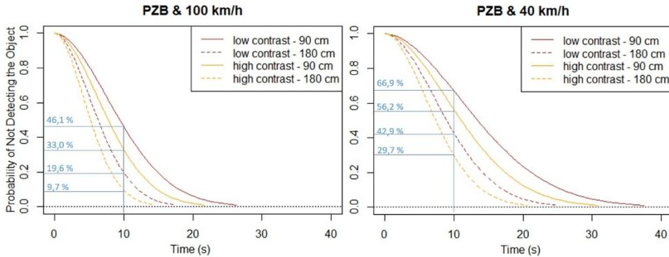
**Figure 3:** Survival probabilities (i.e. probability of not detecting the object) in PZB scenario at 100 km/h and 40 km/h.
