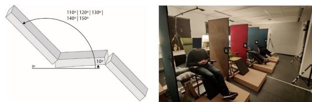
Figure 1: Seat configurations excluding 180^\circ (left) and a research setup impression (right). The leg rest moves parallel to the backrest and the lights were dimmed during the test as they are brighter for the purpose of this picture.
