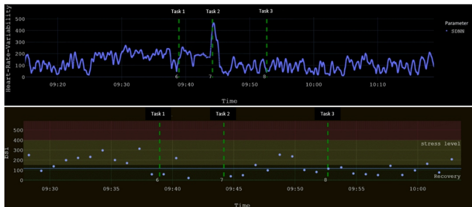
Figure 2: Display of vital data measurements (SDNN) and calculated variables (bsi) showing different levels of strain depending on different activities used as a basis for displaying the traffic light chart.
