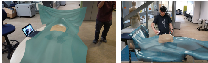
Figure 5: The view from the AR goggle of the virtual bed with the physical simulated cavity.
