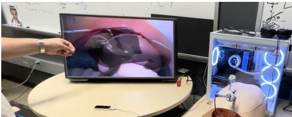
Figure 4: The live laparoscopic video is overlaid with CT 3D liver model by hand tracking.
