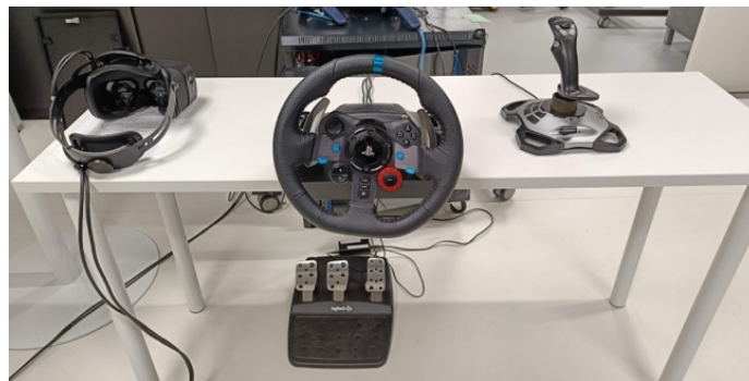
Figure 4: Setup of the first prototype. From the left, there are the Varjo XR-3, Logitech G29 steering wheel and pedals, and Logitech extreme 3D.
