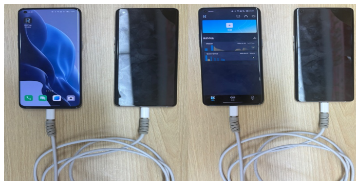
Figure 1: Devices A and B that transmit vibrations through a data cable.
