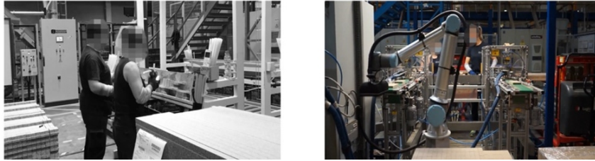
Figure 1: Assembly workstation before (on the left) and after (on the right) HRC implementation.
