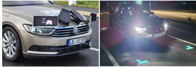
Figure 1: Types of eHMI signals provided by the self-driving car. Left: a luminous hourglass was shown on front displays. Right: a safety zone was shown onto the ground.
