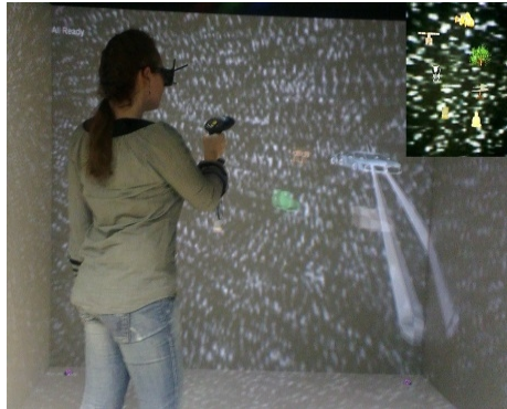
Figure 1: CAVE virtual reality system and the typical scene view (in the upper right corner).
