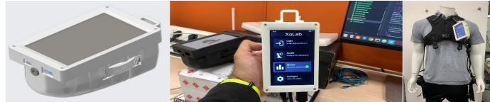
Figure 1: User command interface system. The UCI is a wearable gadget that fits in the palm of the hand and is attached to the exoskeleton.
