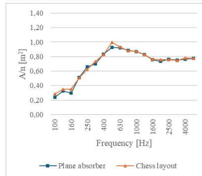
Figure 4: Equivalent absorption area per panel A/n of elements under test with different arrangement modes (matrix and plane absorber installation type “A”) for 80% reverberation chamber occupancy compared to the maximum occupancy made.
