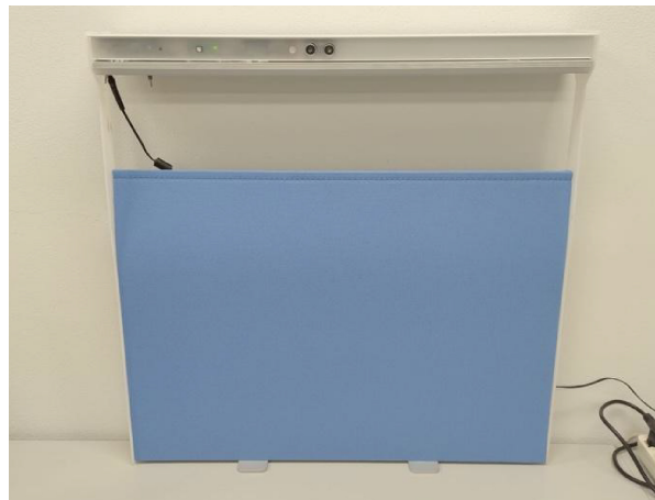
Figure 6: Prototype with sensors inserted into the ALL-LED extruded profile, with the addition of a LED strip for lighting.
