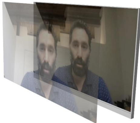
Figure 4: Two displays, one transparent and one opaque, are layered in configuration to produce greater depth (depth not to scale).
