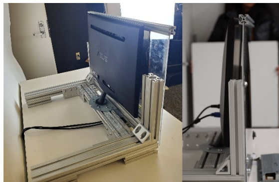
Figure 3: DS-LCD prototype viewed from side and rear.
