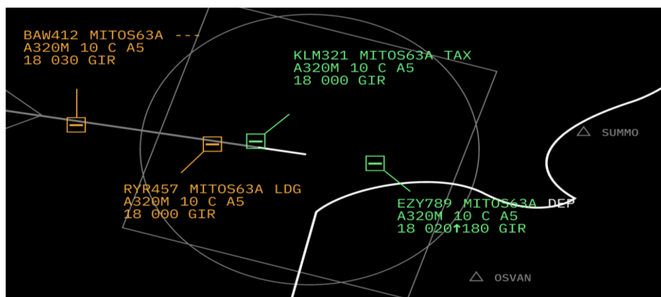
Figure 5a: Extract of tower controller’s HMI showing aircraft positions in real time.
