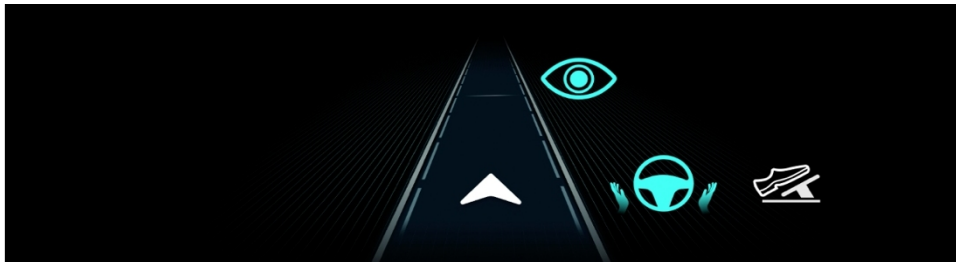
Figure 2: Design A (icons detail, icons parallel to road, road mark lines, animated action).
