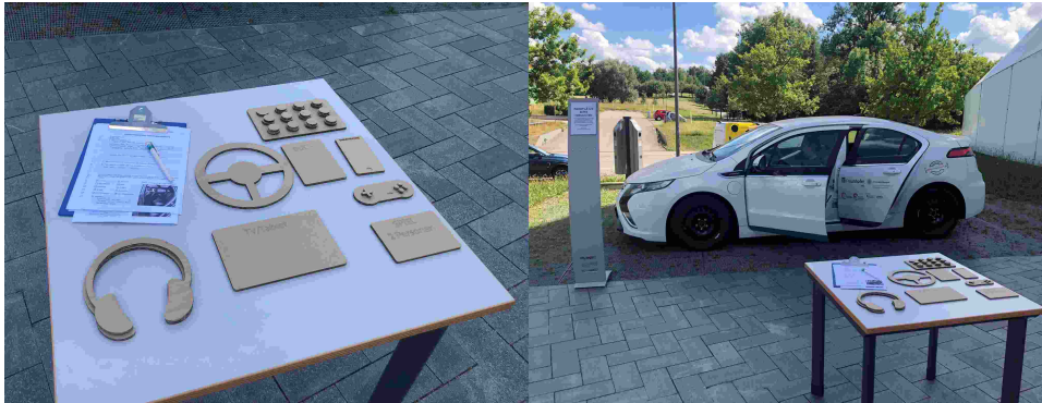
Figure 1: Set up of the Guerrilla testing with paper prototypes and test vehicle.
