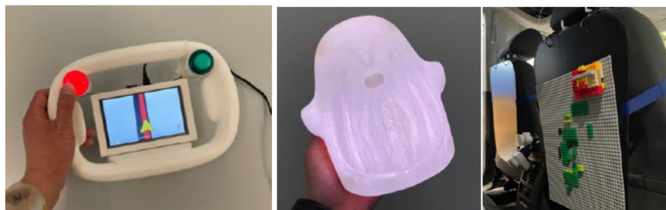
Figure 4: Examples of the prototypes (from left to right): steering wheel connected to the navigation system; glowing night light penguin; playable surface on the back of the seats.
