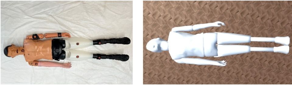
Figure 3: Left: manikin with sensors; right: virtual avatar representing the avatar in the MR glasses.
