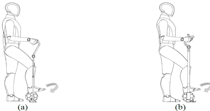
Figure 4: Standing experiments with one leg rolling a ball in clockwise direction for 5 rounds using small quad (a) and ostrich locomotion-inspired cane (b).
