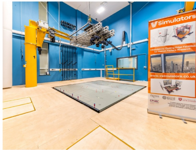
Figure 2: VSimulator rigid platform within an 8 m cube purposely built to accommodate the facility built by The University of Exeter at Exeter Science Park.
