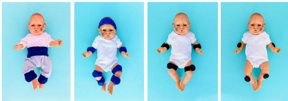
Figure 2: Different sensor attachment systems in form of simple mock-ups (e.g., sensor trousers, stretch bands, stretch Velcro straps, adhesive pads etc.).
