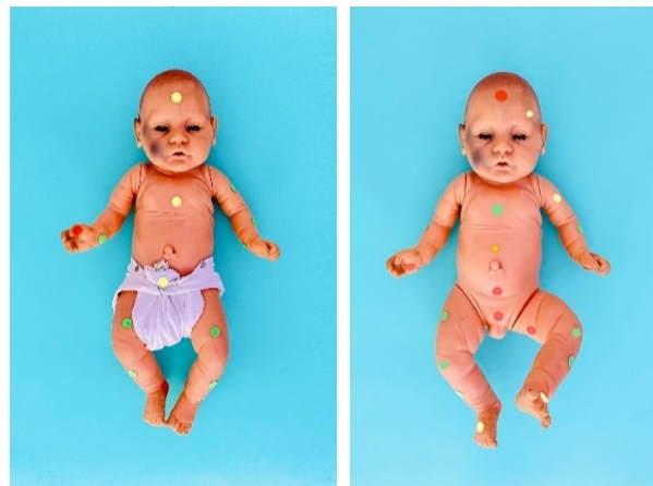
Figure 3: Sensor positions marked by experts (left) and parents (right) for attaching the IMUs (green – recommendation, yellow – acceptable, red – avoid).
