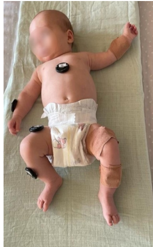
Figure 4: Measurement setup - infant with IMUs attachment with hydrogel adhesive strips (right) and self-adhesive bandages (left) on the sensor mat).
