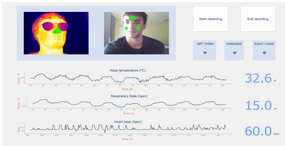
Figure 4: The developed application performs the recording of the different metrics. In the illustration, the nose tip temperature (32.6°C), respiration rate (15 respiration per minute), and heart rate (60 beats per minute) are visible. The application also displays a live video feed from the thermal and RGB cameras.
