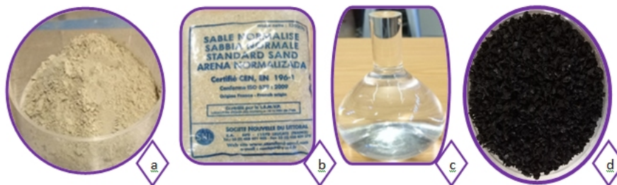
Figure 1: The materials used for the production of mortar (a) 52.5N ordinary portland cement (b) standard sand (c) portable water (d) rubber crumb treated with NaOH.
