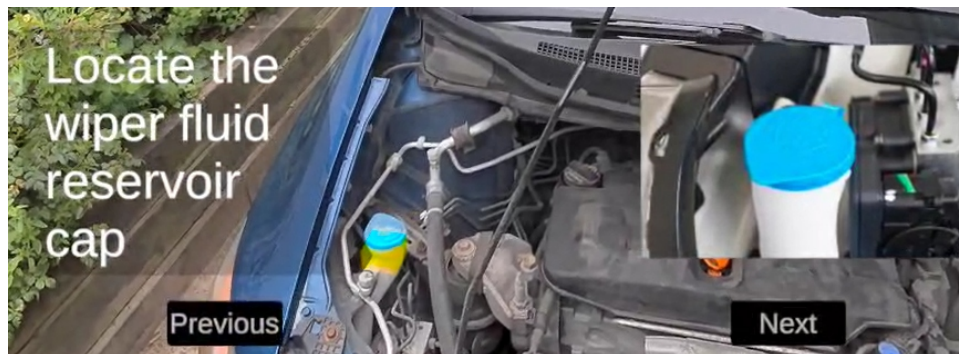
Figure 3: A mixed reality overlay (yellow block) indicating the real location of the reservoir cap on the car, as well as a 2D image of a reservoir cap.
