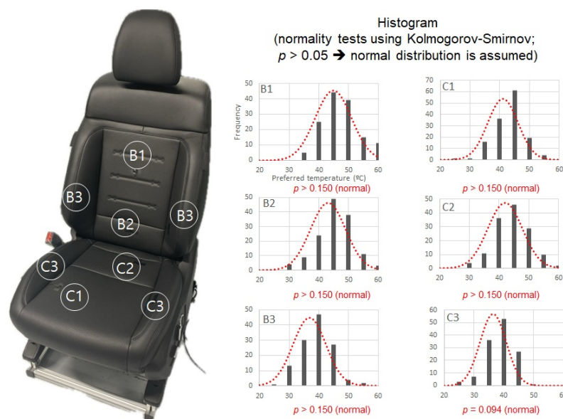
Figure 4: Normal distributions of the preferred temperatures for the six areas of the heated seat.
