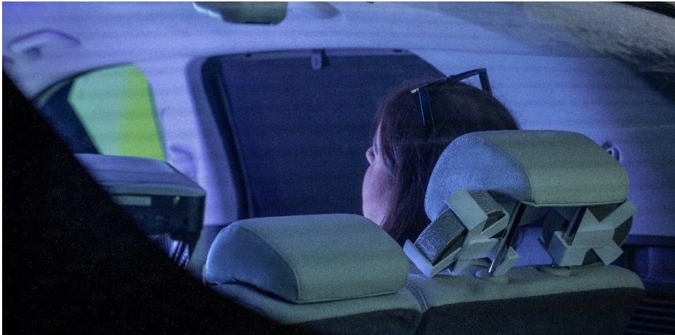
Figure 3: Speakers along the headrest for 360-degree sound experience.
