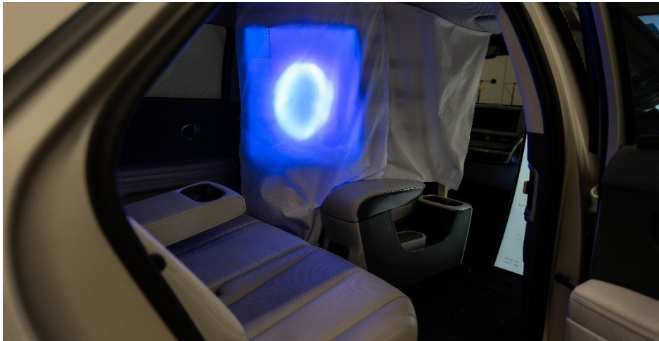
Figure 2: Integrated LED panels in the test vehicle.
