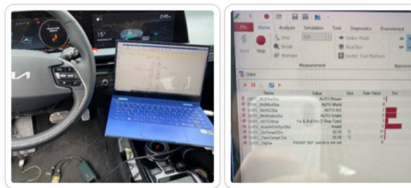
Figure 2: Climate control system signal confirmation using CANoe equipment.
