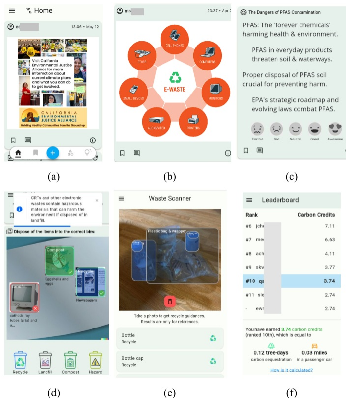
Figure 1: The Waste Genie application. (a) The homepage; (b) A user-created post; (c) An AI synthesized post; (d) An AI-generated quiz, the AI-guidance will be given when a user makes a mistake; (e) The waste scanner; (f) The leaderboard of virtual carbon credits.
