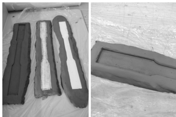
Figure 3: “Dog-bone” specimens made with clay molds.
