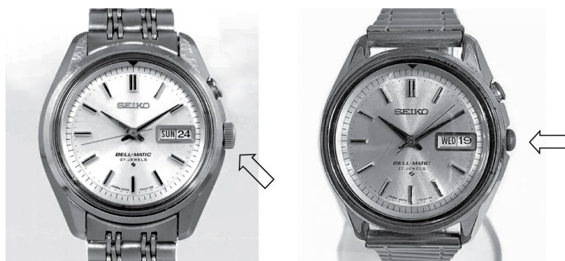
Figure 2: Comparison of the Bell-Matic's crown and bell button. The stainless-steel model (left) shows minimal wear compared to the gold-plated version (right), which exhibits pronounced wear on its crown.
