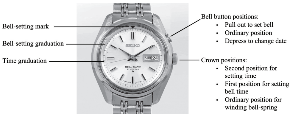
Figure 1: Diagram of the user interface layout and operational instructions. Instructions sourced from an original 1960s Seiko Bell-Matic user manual.
