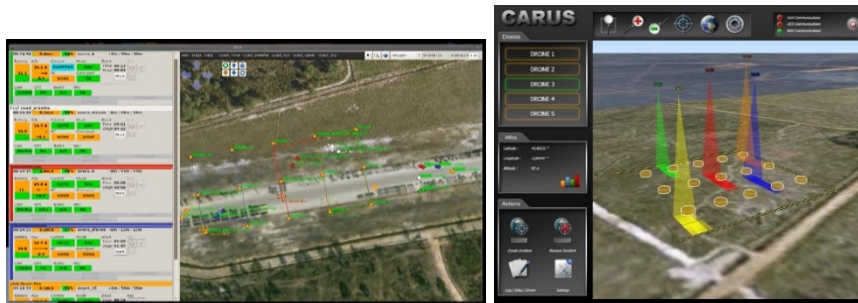
Figure 5: Ground control station, extended to support a swarm of drones (CARUS).
