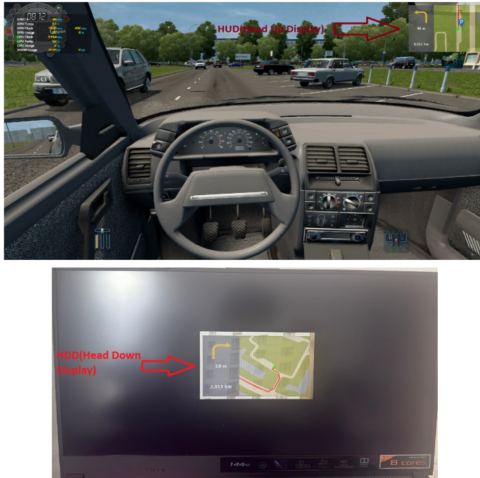
Figure 2: Illustrating HDD and HUD system interface.
