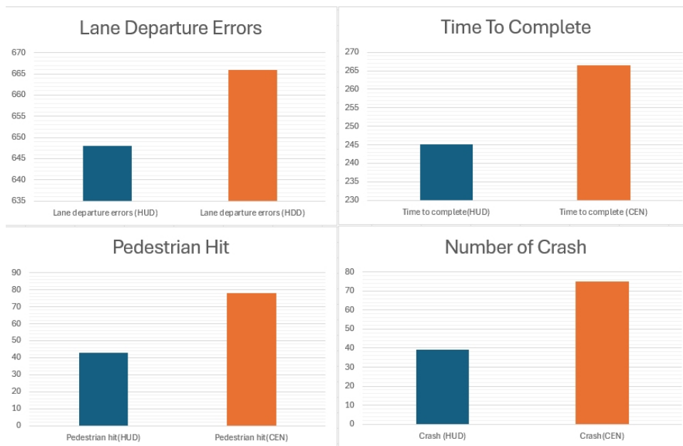
Figure 5: Bar chart demonstrates lane departure errors, Time to complete, pedestrian hit and number of crashes parameters between HUD and HDD.
