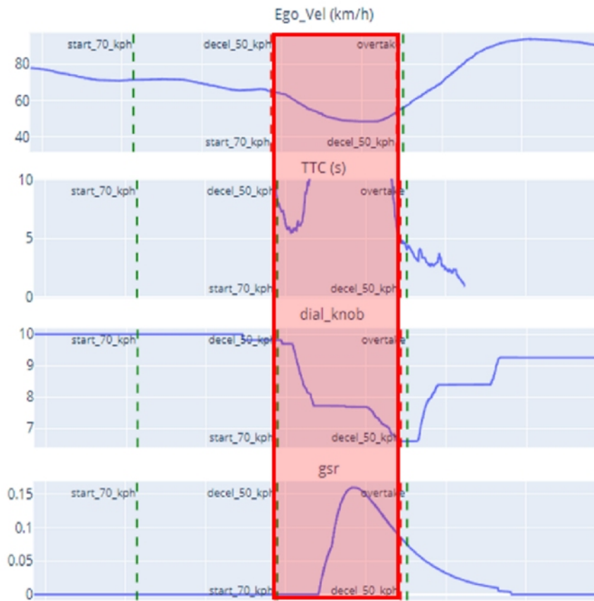
Figure 7: Time-aligned metrics (top to bottom): ego vehicle velocity, TTC, subjective dial knob score and GSR. The red area indicates the time interval of the deceleration scenario.
