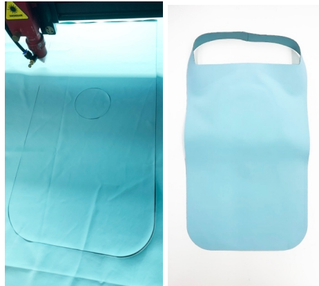
b. The water bag is made of laser-cut high-density nanofiber membrane
