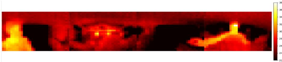
**Figure 3:** View from the thermal camera array, showing an unprocessed image with one passenger seated in the rear left seat and another passenger occupying the left seat in the last row (self-created).
