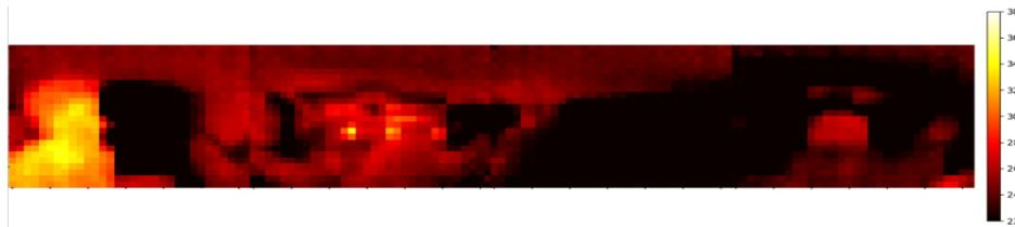
**Figure 2:** View from the thermal camera array, showing one passenger seated in the rear left seat (self-created).
