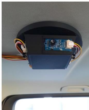
**Figure 1:** Camera array mounted on the interior roof of the cabin (self-created).
