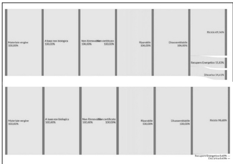
Figure 1: Graphic representation of the material circularity performances of the two solutions, in reinforced Nylon (top) and Zamak 15 (bottom), on the input and output flows of materials obtained with the Circulartool software by Matrec.
