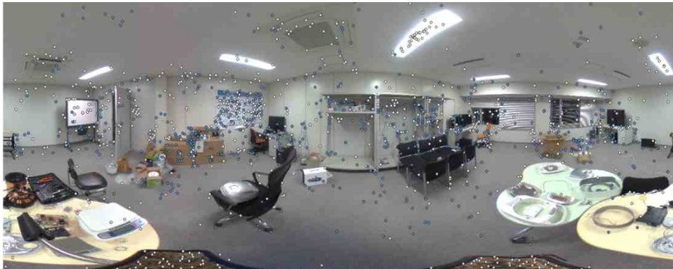
Figure 2: Feature point detection and matching among spherical images.
