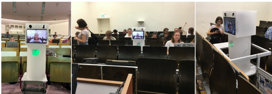
Figure 3: Functional prototype of the Fernstudent in the lecture hall during the field test.
