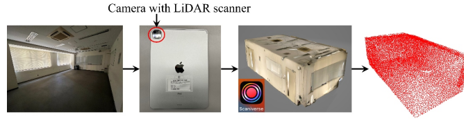
Figure 6: Flow from acquisition to sampling of indoor spatial point cloud data.
