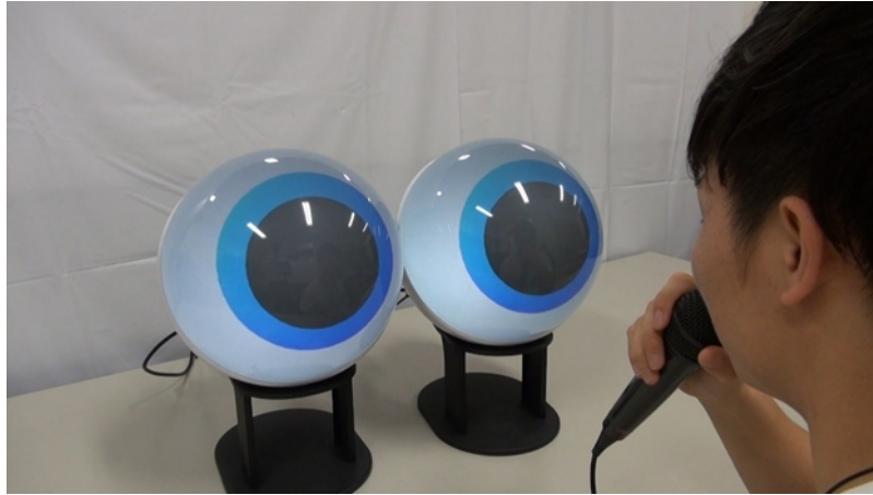
Figure 1: Pupiloid: pupil response robot (reference: Sejima, 2025).
