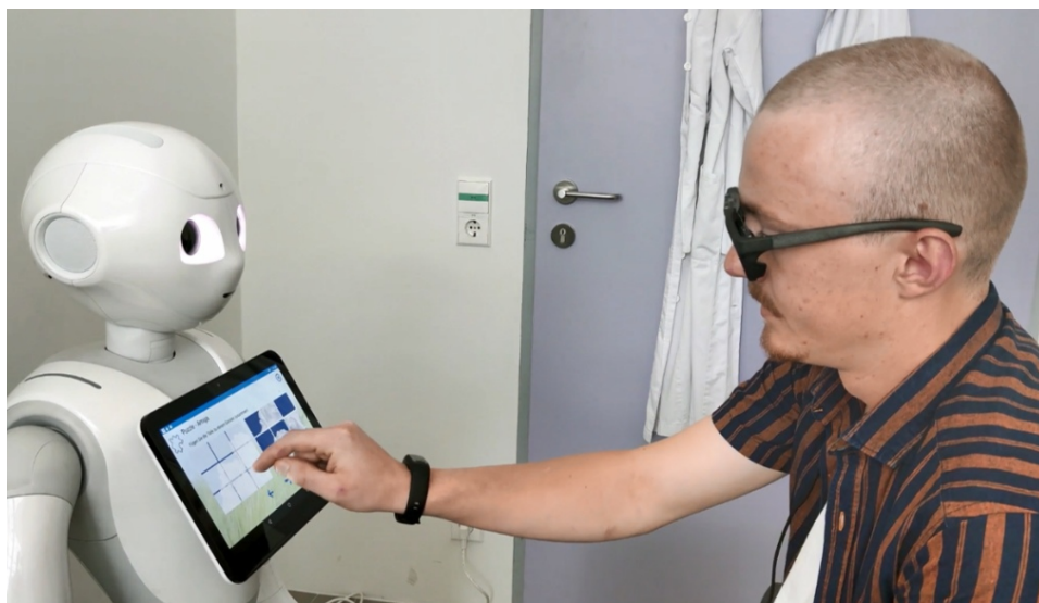
Figure 5: AMIGA system in the field test on the premises of the psychiatric clinics of the Medical University of Graz. The participant interacts with the tablet-supported cognitive training on the socially assistive robot pepper, as well as human factors-supported evaluation with wearable biosignal sensors (on the wrist) and eye tracking glasses.
